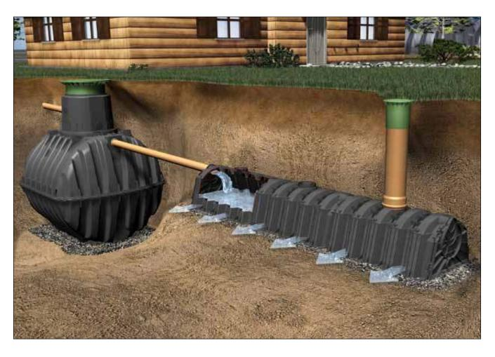
The Graf Infiltration Tunnel has been mainly designed for the use in private and rural areas. The system which consists of one or several tunnel modules and two end plates can be extended at will. The laying is realized in one or more lines of the same level. As the weight of one module is only 11 kilos, the handling of the Infiltration Tunnel is
