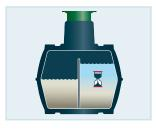
3. Rest phase A rest phase now follows, during which the live sludge sinks to the bottom of the system. This allows a clarified water zone to form at the top of the SBR reservoir.
